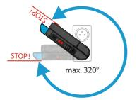
The receiver can be rotated by a maximum angle of 320° around its XLR-3 connector.
