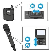
Both the bodypack transmitter and the SKM AVX-S handheld transmitter have a Mute switch that mutes the audio signal without switching the transmitter off.
