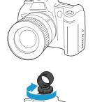
Fasten the hot shoe adapter using the locking screw.
