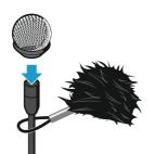
Carefully stretch the opening of the fur windshield and slide it over the metal windshield. Make sure that the fur windshield completely covers the metal windshield.
