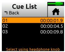
2. Tap Move and rotate the HP encoder to adjust the selection in 0.1 second increments.
