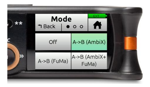
When Ambisonics Mode is enabled, input channels 5-6 (MixPre-6) and 5-10 (MixPre-10T) are no longer available and input channels 1-4 are automatically linked so that channel knob 1 becomes the master gain control for those four channels.
