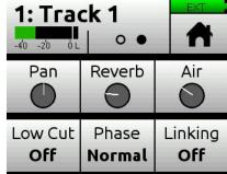
Each Channel screen provides two pages of settings—indicated by Dots icon. Tap the Dots icon to switch pages.
